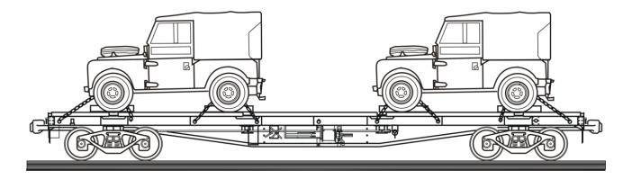
12. You will note that they have been positioned so that the front wheels of one Landrover and the rear wheels of the other Landrover have been positioned over the center of the bogie bolsters.
